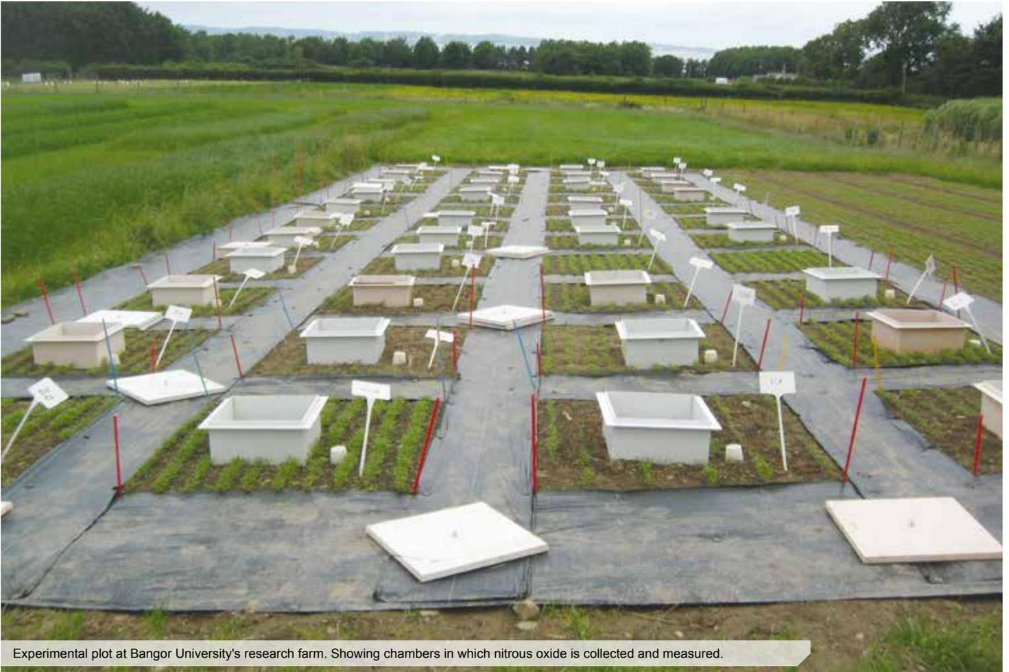
Experimental plot at Bangor University's research farm. Showing chambers in which nitrous oxide is collected and measured.
